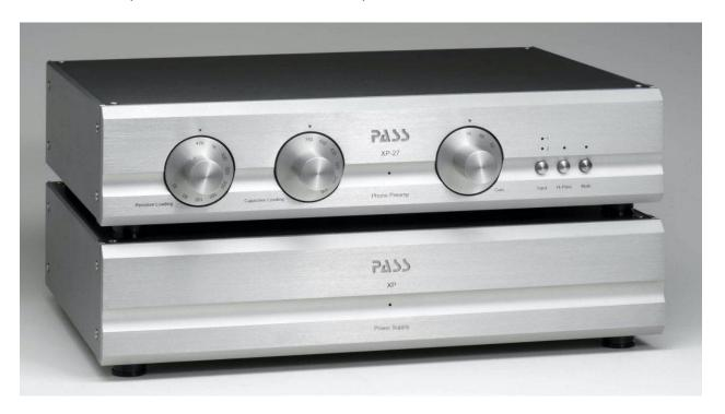
The new design uses double-shielded, low-noise toroidal transformers in an external supply, connected via aviation-grade circular connectors using silver over oxygen-free copper. The power supply is dual mono with two transformers with lower radiated and mechanical noise. Noise is the most prominent part of THD+N at low levels, so by lowering noise we get better resolution and dynamics.
